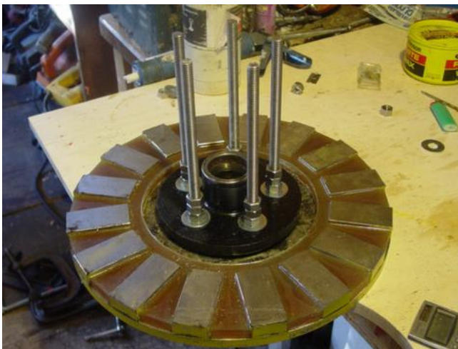
One Magnet Rotor Mounted to Hub Jacking Screws Extend Up to Mount And Adjust The Opposite Rotor
