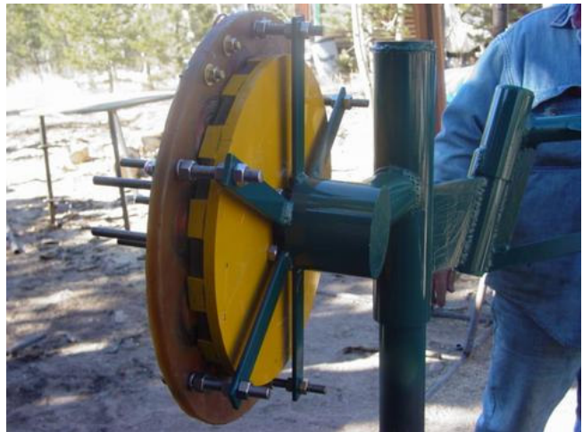
Rotor and Hub Mounted on Tower Head Stator is in Position in Front of The Rotor
