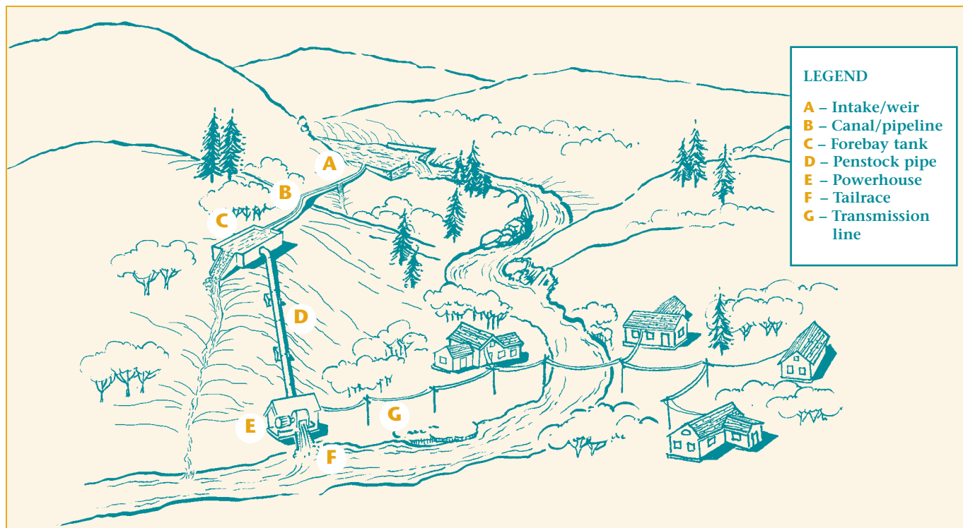
Figure 2. Principal components of a micro-hydropower system
