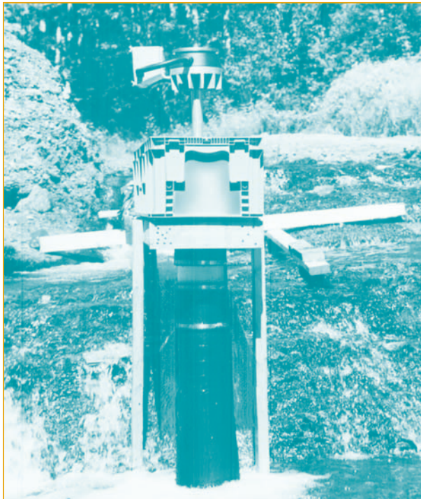
Figure 23. A 1-kW rated low-head battery-based system (photo courtesy of Energy Systems & Design)
