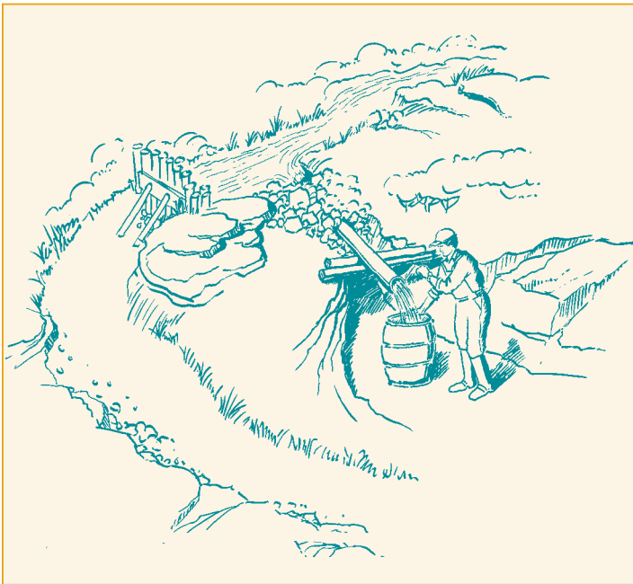
Figure 35. Measuring water flow rate using container method
