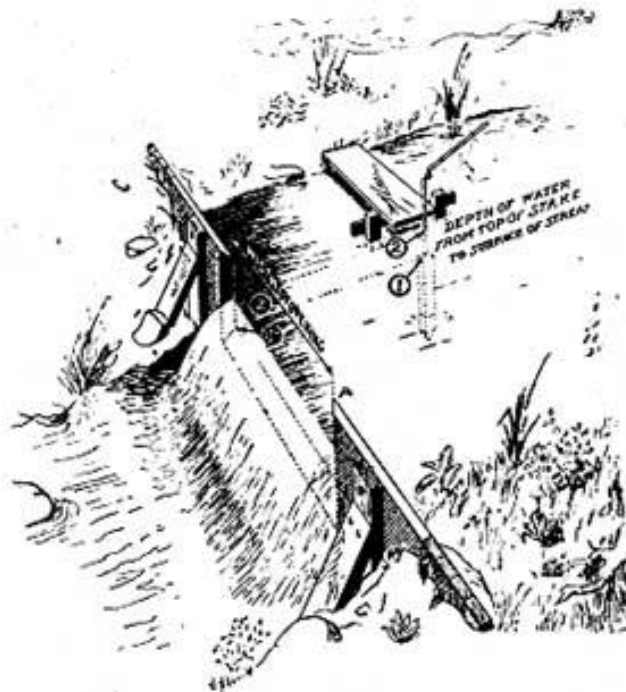
A WEIR FOR MEASURING THE FLOW OF A SMALL STREAM
